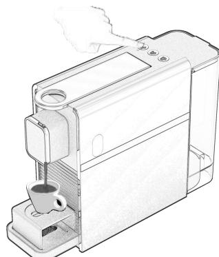
**5** Once the desired amount of coffee has been obtained, then releasing the button to stop supply.
