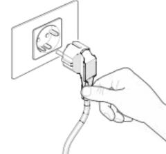
**4** Fit the supply plug into the power outlet.
