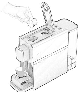
**3** Lower the capsule loading lever to close the capsule fitting compartment.
